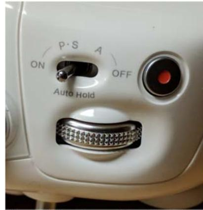
Figure 2. Function mode switch, video record button and gimbal control wheel. Will be controlled with your left
