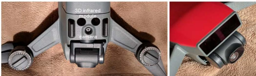
Figure 1. Vision System of dji Spark, with (left) downward-looking 3D infrared module and camera, and (right) the forward-looking 3D sensing system.
