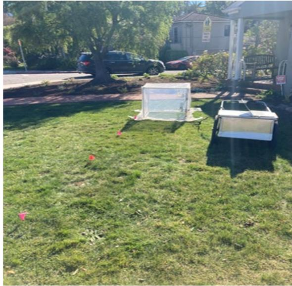
Figure 2. An example of the pilot study sampling method showing the chamber during observation. Pink flags indicate the remaining four sample plots along the lawn transect.
