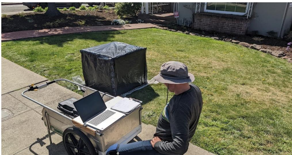
Figure 4. An example of the darkened closed chamber connected to data logger and laptop used to measure ecosystem respiration on Lawn A.
