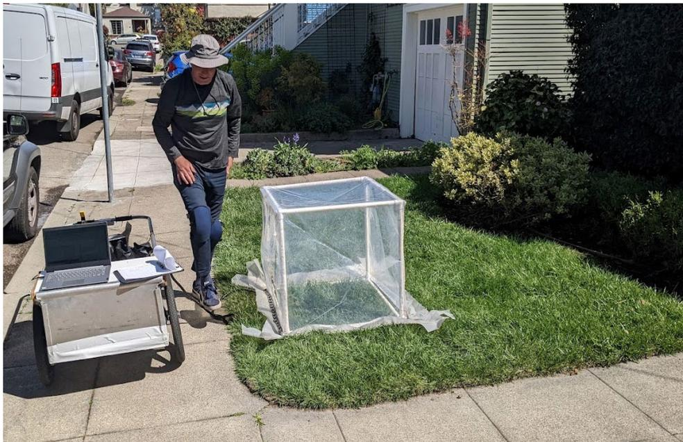
Figure 5. An example of the transparent closed chamber connected to data logger and laptop used to measure CO<sub>2</sub> concentration in Lawn B. (Photo: Andrew Oliphant)
