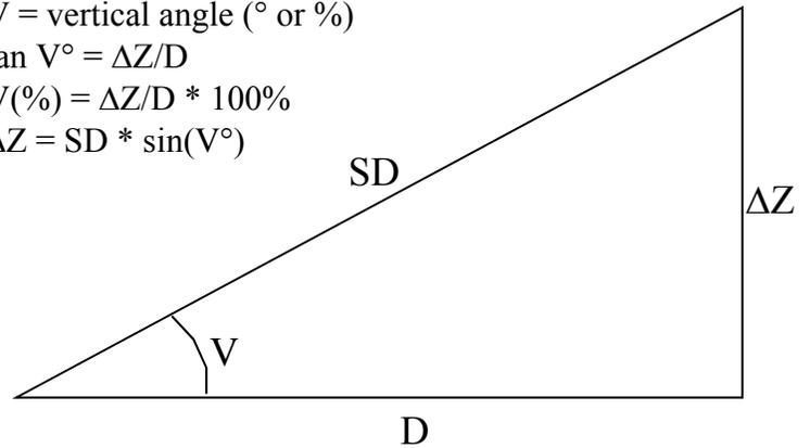
Fig. 4. Vertical angle relationships and equations.
