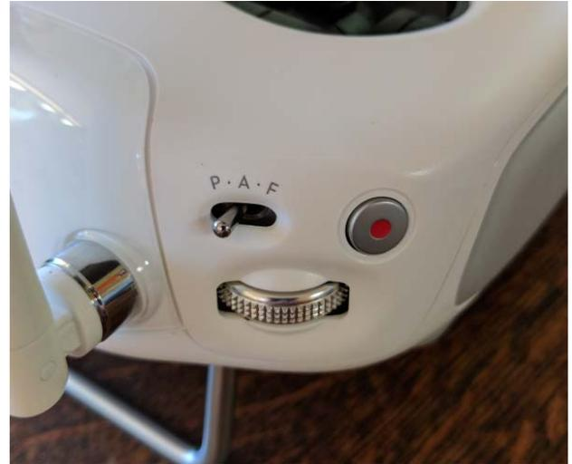
Figure 3. Function mode switch, video record button and gimbal control wheel. Will be controlled with your left hand.
